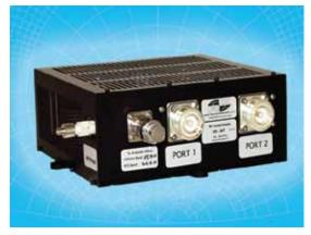
The Model HD-A37 is a 3 dB Hybrid assembly with an integral high power low PIM termination, a continously adjustable attenuator, and a calibrated fixed monitor output port. The assembly combines input Tx power and provides a highly attenuatored adjustable output to feed
